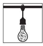
**STEP 2: ASSEMBLE** With light string un-plugged (no power), insert provided A19 Bulbs into each socket and gently tighten clockwise until fully seated in rubber seal. Do not over tighten.
